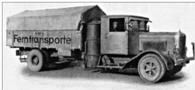
German wartime Henschel truck with Imbert producer-gas generator behind the driver's cabin.
